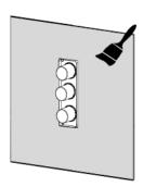
Create a dry wall around the installation box and brush with water proof glue.
