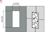
Leave a hole on tile covering according to chart dimensions and real product size. Use silicone along the installation box to seal. 09
