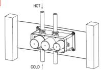
Connect hot and cold water pipes and all outlets accordingly and test the leakage.
