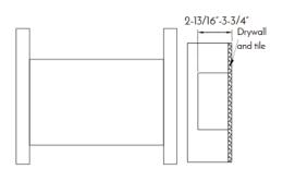
Fix a wood plate to the two wood pipes for faucet installation.
