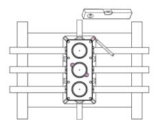
Put the installation box on the wood plate. Measure the correct position with level and marks.
