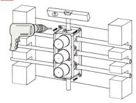
Screw the installation box to the wood plate.
