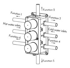
Design the pipelines connection inside the wall accordingly to the function chart.
