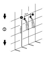
Flush the water supply lines throughly to drain debris and impurities. Shut off the water before installation.
