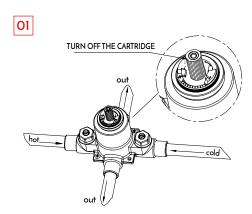
Make sure all inlets  $\alpha$  outlet pipe were well connected, and the valve is closed.
