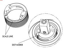
After remove the temperature adjust component you can see there is eleven scale line on the temperatue adjust component, and there is a dotmark on the cartridge.
