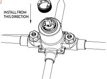
When the 1st scale line near the "+" sign be alignwith the dot mark on cartridge, the water temperature wold be the highes. If the 2st scale line near the "+" sign be alignwith the dot mark, the fixed highest temperature would be reduce accordingly. In turn, when the 1st scale line near to "-" sign align with the dot mark, the lowest temperature is set By using the temperature adjut component, you can limit the highest temperature of the pressure balance valve.
