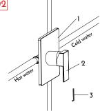
Fix the body assembly and water lines in the wall. Put the deck plate (1), and then put the handle (2) on the handle base and tighten the screw with allen key (3).
