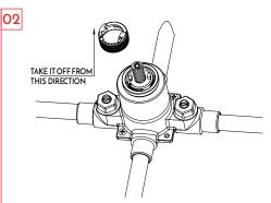
Then take off the temperature adjust component. Please notice there is no need to remove the olve body, but by using a tool (such as a "\_" screwdriver) to pry up the temperature adjust component directly
