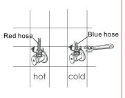
Water-supplying value (left to hot water and right to cold).
