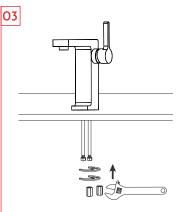
Put all hose through the plastic gasket (6) the through the metal gasket (7), finally screw the nut fitting (8), tight in with screw (9).
