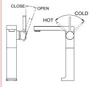
Pull the handle rightward in horizontal to turn on the faucet. Leftward in horizontal line to turn off. Move the hand counterclock wise from cold to hot.
