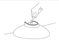
Place the countertop basin on the hole. Ensure it is centered and that there is enough space for it to lay flat. After these verifications, take it back, turn it upside down and apply a generous portion of silicone adhesive under the basin (see illustration 3).
