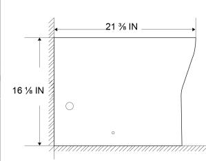
A trap is not supplied with the bidet. For installation of a trap in the floor, provisions must be made.
