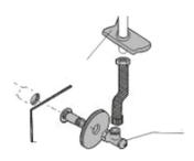
Connect the water inlet to the tank. Make sure water pressure is suffcient to fll the tank.
