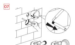
Cut the protection sleeve outside of the wall with a knife. Apply lubricant on joint surface of straight tube and connecting pipe.
