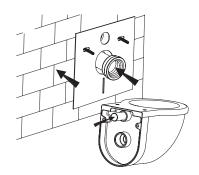
Firstly insert connecting pipe into discharging outlet and straight tube ceramic hole.
