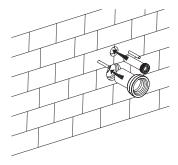
Fully insert the straight tube into de cistern flushing outlet and connecting pipe into discharging outlet.
