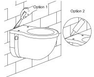
Fill the gap with white cement or glass cement.
