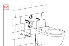
Adjust length of connecting bolt to be d+20mm.
