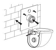
Firstly insert connecting pipe into discharging outlet and straight tube ceramic hole.
