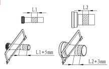
As per drawing, L1 is distance between the two lines on straight tube. L2 is distance between the two lines on connecting pipe. Cut the straight tube and connecting pipe as per above drawing
