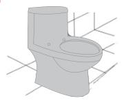
Apply a mould-proof silicon between the foor and the toilet base.
