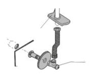
Connect the water inlet to the tank. Make sure water pressure is sufficient to fll the tank.
