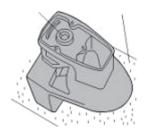
The toilet should be placed on the floor upside down, on a soft piece of cloth to prevent scratching. Place the wax ring in the circular recess in the base of the bowl.
