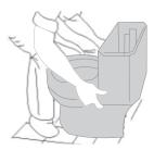
Unplug the waste opening. Gently place the toilet right side up in position with the toilet mounting bolts going through the holes in the porcelain base. Press down on the toilet until it is leveled, if necessary use wedges to make it leveled.
