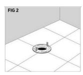
Install new floor bolts into floor flange. (Figure 2)
