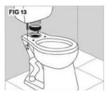
Attach the large rubber sealing gasket to the center drain hole under the tank. (Figure 13)
