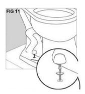
Install plastic cap washers, followed by metal washers and nuts onto the closet-bolts. (Figure 11) Tighten the bolts alternately until toilet is firmly seated on the floor.
