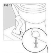
Install plastic cap washers, followed by metal washers and nuts onto the closet-bolts. (Figure 11) Tighten the bolts alternately until toilet is firmly seated on the floor.
