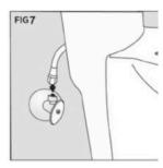
Connect the flexible water supply line (not included) to the shut-off valve. Tighten coupling nut securely (Figure 7).
