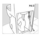
Attach flexible water supply line to the inlet of the fill valve and hand tighten only. At this point, DO NOT connect to the water shut-off valve. (Figure 3)
