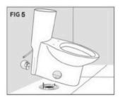
Lower the toilet onto the closet bolts, so the bolts project through mounting holes in base of toilet. (Figure 5) Using a rocking motion, press the bowl to position the toilet onto de flange.
