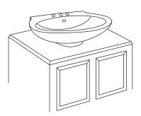
Choose the location on the vanity top where you will install the countertop basin. Make sure there is enough space under the counter for the water lines and the drain. Also, ensure that the space between the back of the basin and the backsplash (or the wall) is large enough for the faucet. 02
