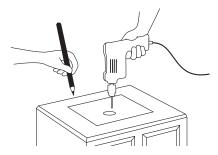
Confirm that the mark on the vanity lines up with the basin you have chosen and that it is centered. Then cut the hole the size of the pipe (see illustration 2).
