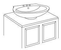
Choose the location on the vanity top where you will install the countertop basin. Make sure there is enough space under the counter for the water lines and the drain. Also, ensure that the space between the back of the basin and the backsplash (or the wall) is large enough for the faucet.
