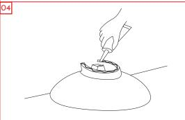
Place the countertop basin on the hole. Ensure it is centered and that there is enough space for it to lay flat. After these verifications, take it back, turn it upside down and apply a generous portion of silicone adhesive under the basin (see illustration 3).
