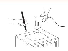
Confirm that the mark on the vanity lines up with the basin you have chosen and that it is centered. Then cut the hole the size of the pipe (see illustration 2).
