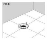
Install new closet bolts into closet flange. (Figure 8) You can pre-cut the closet bolts to the desired length to put on the bolt cap by doing the following: Temporarily install closet bolts and set the toilet and place the washers and nuts onto the bolts. Cut the closet bolts to the length and then turn the toilet upside down onto a soft surface to avoid scratches on the finish.
