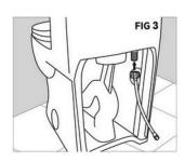
Attach flexible water supply line to the inlet of the fill valve and hand tighten only. At this point, DO NOT connect to the water shut-off valve. (Figure 3)
