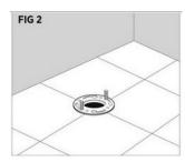
Install new floor bolts into floor flange. (Figure 2)
