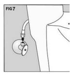
Connect the flexible water supply line (not included) to the shut-off valve. Tighten coupling nut securely (Figure 7).
