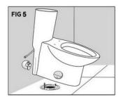
Lower the toilet onto the closet bolts, so the bolts project through mounting holes in base of toilet. (Figure 5) Using a rocking motion, press the bowl to position the toilet onto de flange.
