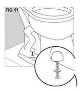
Install plastic cap washers, followed by metal washers and nuts onto the closet-bolts. (Figure 11) Tighten the bolts alternately until toilet is firmly seated on the floor.
