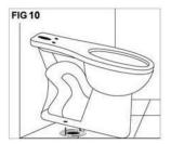
Lower the toilet onto the closet bolts, so the bolts project through mounting holes in base of toilet. (Figure 10) Using a rocking motion, press the bowl down to position the toilet onto the flange.
