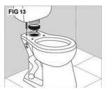
Attach the large rubber sealing gasket to the center drain hole under the tank. (Figure 13)
