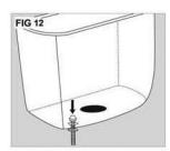
Insert tank bolts inside the tank. Use the metal and rubber washers supplied to create a seal. (Figure 12)
