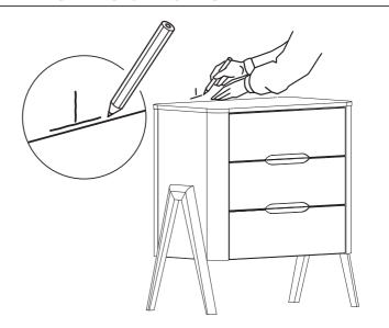
2. Attach fixing strap supplied to position on wall as shown. Ensure correct screws and fittings as appropriate to the type of wall are used. Check the wall is suitable for attaching this furniture.
