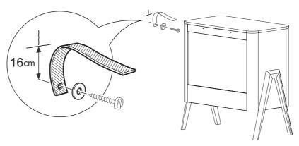
3. Using the wood screw and washer supplied attach fixing strap to the underside
