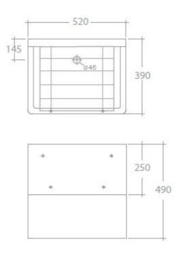
\* DUE TO THE MANUFACTURING PROCESS SINKS MAY HAVE SLIGHT VARIANCES IN SIZE. THESE DIMENSIONS SHOULD BE USED AS A GUIDE ONLY. WE STRONGLY RECOMMEND THE SINK BE ON SITE WHEN CABINETS OR BENCH TOPS ARE BEING PREPARED FOR THE SINK.
