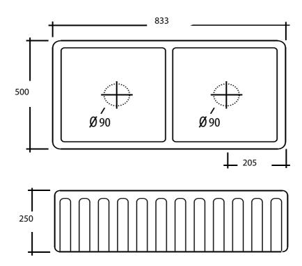
\* DUE TO THE MANUFACTURING PROCESS SINKS MAY HAVE SLIGHT VARIANCES IN SIZE. THESE DIMENSIONS SHOULD BE USED AS A GUIDE ONLY. WE STRONGLY RECOMMEND THE SINK BE ON SITE WHEN CABINETS OR BENCH TOPS ARE BEING PREPARED FOR THE SINK.
