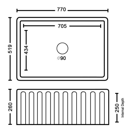
\*DUE TO THE MANUFACTURING PROCESS SINKS MAY HAVE SLIGHT VARIANCES IN SIZE. THESE DIMENSIONS SHOULD BE USED AS A GUIDE ONLY. WE STRONGLY RECOMMEND THE SINK BE ON SITE WHEN CABINETS OR BENCH TOPS ARE BEING PREPARED FOR THE SINK.
