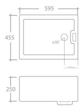
\* DUE TO THE MANUFACTURING PROCESS SINKS MAY HAVE SLIGHT VARIANCES IN SIZE. THESE DIMENSIONS SHOULD BE USED AS A GUIDE ONLY. WE STRONGLY RECOMMEND THE SINK BE ON SITE WHEN CABINETS OR BENCH TOPS ARE BEING PREPARED FOR THE SINK.
