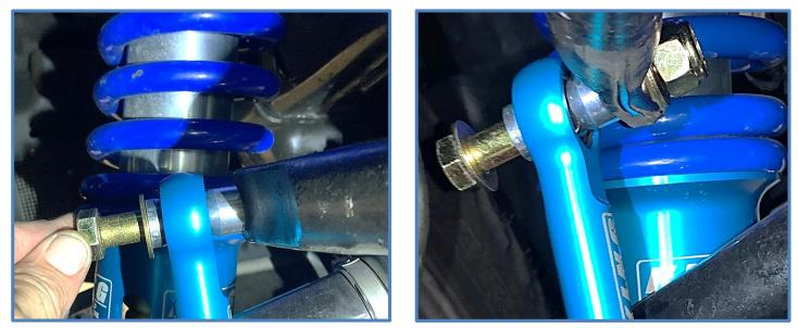
5. Install the provided 14mm X 80mm Bolt (CB3836) with washer (CW1751) through the sway bar link and into the sway bar mount on the lower control arm so that the longer spacer is facing the sway bar mount and the nut will be on the back side of mount. Install a washer and nut (CN3007) and thread nut on finger tight for now.
