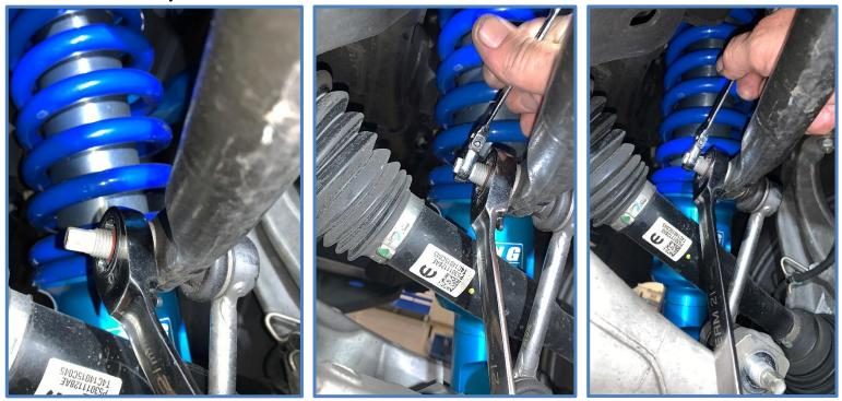
3. <u>Install King Sway Bar Links</u> - Make sure to install links with spacers facing the correct way. Follow the install guide for proper orientation. Failure to install links as shown may cause damage to product and/or vehicle.
