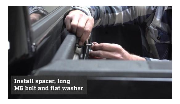
Position a spacer behind the MOLLE panel, then take an M6 bolt, add a flat washer, and thread it into the factory bed hole and hand tighten it. Repeat this process for each of the remaining holes.
