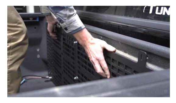
With the bed prepped, you can now position the MOLLE panel into place. Be sure to line-up the holes with the brackets facing outwards.
