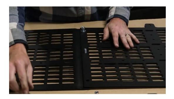
Next, grab a 3/8" bolt, add a washer, and insert it through from the bottom side of the panel. Finish by adding a flat washer and a locknut. Repeat this process for each of the three bolts, making sure to only hand-tighten them for now.
