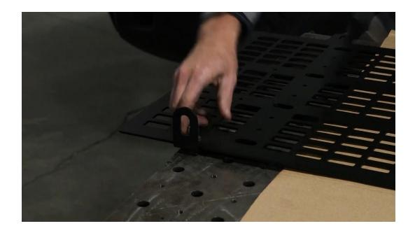
Now, we'll install the brackets. Position the first as seen in the above image. Then, take a 3/8" bolt, add a washer, and slide it through from the back-side. Add a flat washer and a lock nut, and then hand-tighten it down. Repeat this same process for the other side.
