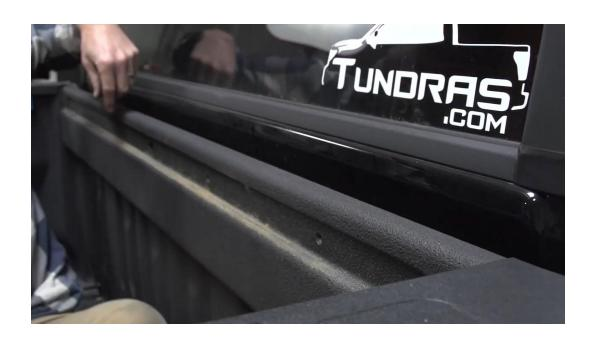
If you have the factory accessory rail on the back of your bed, there are 4 additional bolts to remove. If you don't, then you'll move on to the next step, which is to remove the rear bed bolts. For this, you'll use a T55 Torx.
