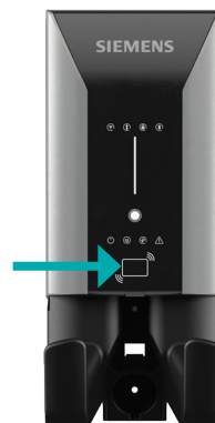
RFID on Versicharge commercial units provide secure hands-free ability to pay-to-charge.
