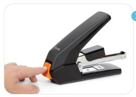
Place the stapler on a flat surface. Press down on the orange button labeled "PUSH" located on the back of the stapler. This will cause the stapler slide mechanism to release and jut out. If needed, pull the stapler slide mechanism out all the way until it catches to provide more room to insert staples.
