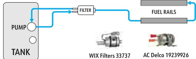
EFI Fuel line routing using an adjustable fuel regulator before the fuel rails.
