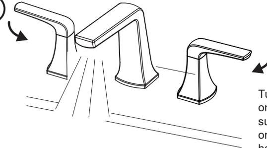
Turn the faucet handle all the way on, turn on hot and cold water supply and flush water lines for one minute. Reinstall aerator by hand.
