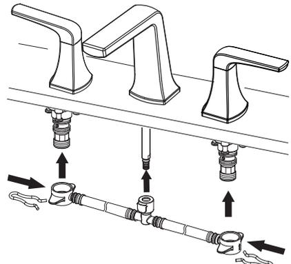
Position the flexible hose and fix it to the faucet as shown with clamp spring.
