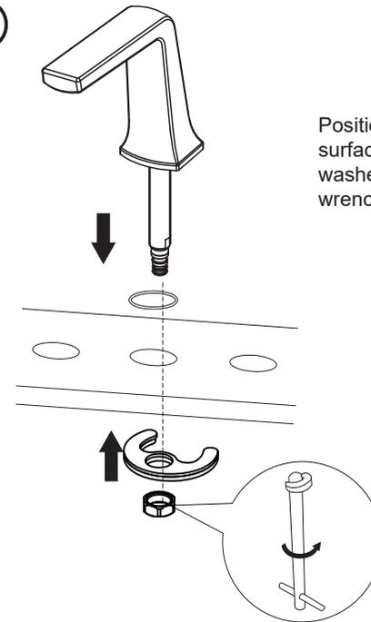
Position the body with o-ring on the installation surface as shown and secure it with metal washer and tighten the lock nut with basin wrench.
