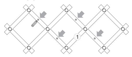
Drill small pilot holes into the wall at the marked locations and insert plastic anchors.
