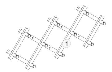
To affix the item to drywall, determine final placement on the wall, and mark the keyhole opening placement on the wall with pencil. Be sure to confirm precise distance and levelness between holes for accurate hanging.
