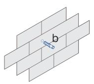
Attach the coat rack to the anchors with screws. Tighten with a phillips screwdriver.
