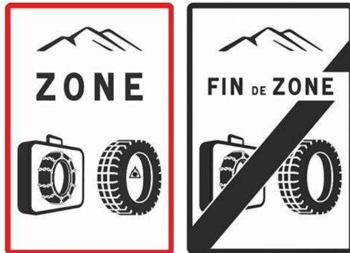
The new road signs B58 and B59 signaling beginning and end of winter equipment sections
