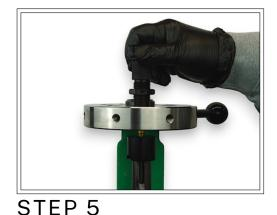
Turn the die down. When the tip makes contact with the floor of the case tighten the die down a 1/2 turn.
