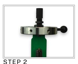
Place the swage onto the ram.
