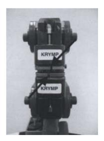
**19,** When the shrinker / stretcher machine is not in use, the securing pin has to be mounted to avoid injuries.
