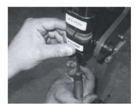
**18,** It is very important to use the same type of jaws, shrinker / shrinker jaws together and stretcher / stretcher jaws together.
