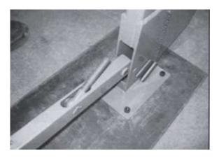
**7,** Move the foot pedal in to the main unit and at the same time, with your other hand guide the threaded link screw up in the opening.
