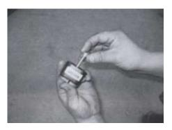
**17.** Then place the jaw one at a time with the text to the outside. Then use the wrench to tighten the jaws.
