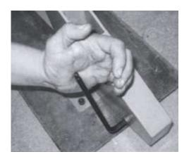
10, Now mount the spring , first onto the main unit, then to the foot pedal.
