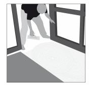
which consists of applying the adhesive on both the substrate and the back of the tile, in order to ensure a 100% contact with the bonding material.
