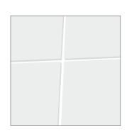
8. The grouting material should be applied 24/48 hours after the covering application, order to help evaporation of the water used prepare the bonding mixture. This way is possible to avoid moisture stains that might end causing up efflorescence pathologies.
