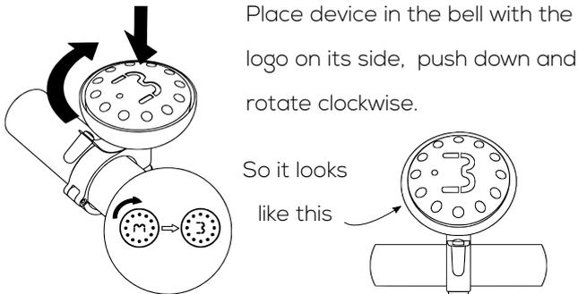
To take out: rotate anti-clockwise until the device pops out of the bell mount.
