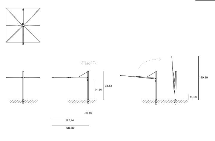
In combination with the permanent fixation & pole extension
