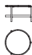
77025 Tavolino rotondo, top frassino Round low table, top in ash wood Ø cm 56 x h 34 Ø in 22 x h 13 3/8
