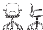
5-spoke base with castors and armrests L 66 P 66 H 82/89 cm W 26" D 26" H 32 2/8 /35"
