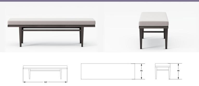
$\textbf{INTERNAL CONSTRUCTION:} \ Solid \ Iroko \ frame, \ mortice \ and \ tenon \ joined. \ Attached \ attached \ upholstered \ seat \ cushion. \ All \ exposed$
