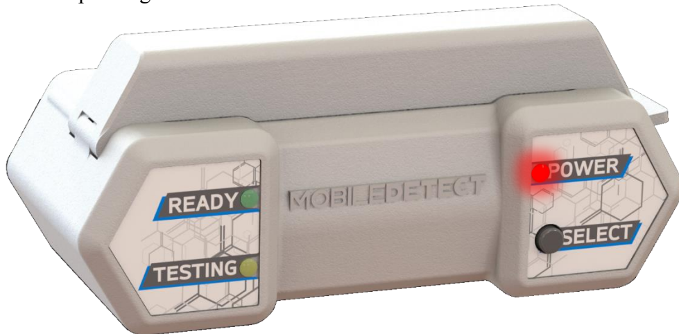
Figure 3: MD-Bio BCC19 Heater in Standby Mode
