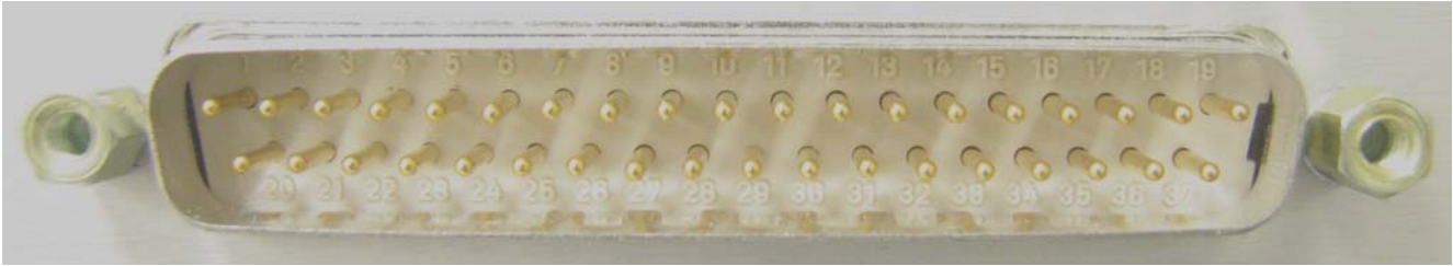
P101 Autopilot Rear Connector (Viewed from rear of autopilot) or wire side of connector.
