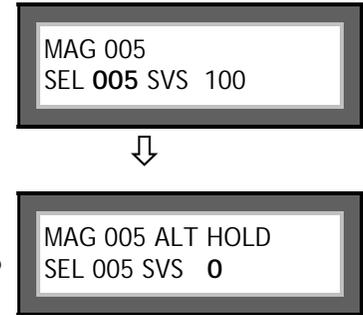
In both cases, the selected heading will be underlined on the bottom left of the display, and the autopilot will be in the altitude hold mode. Both the pitch and roll servos should stop, or move only very slowly.
