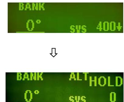
In both cases, the selected heading will be underlined on the bottom left of the display, and the autopilot will be in the altitude hold mode. Both the pitch and roll servos should stop, or move only very slowly.
