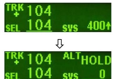
In both cases, the selected heading will be underlined on the bottom left of the display, and the autopilot will be in the altitude hold mode.
