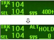
In both cases, the selected heading will be underlined on the bottom left of the display, and the autopilot will be in the altitude hold mode.
