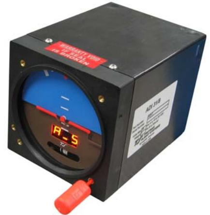
Mounting of the ADI is not angle sensitive as long as the tilt is not more than 10 degrees in any direction, so no shimming is needed for panel tilt compensation. The mounting screws are 6-32 thread with a maximum length of 3/8". Brass screws are preferred.
