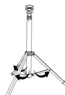
Pull legs outward and set leg stance. Once leg stance has been determined tighten (clockwise) locking knob to set stance.
