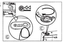
After all the pictures are taken, press the rewind button (G) located at the bottom of the camera. Turn the film rewind crank (C) clockwise until all film is re-wound back into the film canister.
