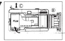
Open the camera back door (B). Lift up the film rewind crank (C), and remove the film for processing.
