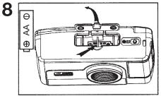
Open the battery door in the direction of the arrow. Insert one "AA "alkaline battery into the battery chamber. Make sure the battery is inserted according to the correct polarity. The correct polarity (the "+" and "-" ends of the battery) is indicated inside the battery compartment.
