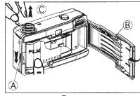
Press the latch (A) in the direction of the arrow and open the camera back door (B). Lift up the film rewind crank (C) and place a new roll of film into the film chamber.
