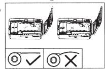
Ensure that the film lays flat against the center of the camera and close the camera's back door.
