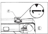
Continue to advance the film by turning the film advance wheel (E) until it stops. Press the shutter button. Repeat this procedure one more time. The Film Counter (F) will now show number "1", and the camera is ready for taking pictures.
