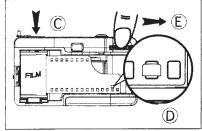
Push the rewind crank (C) back into place. Pull out the film from the film canister and hook the 2nd hole onto the fim take-up spool (D). Slightly advance the film by turning the film advance wheel (E)
