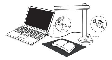
2 . SD-3000NC will connect automatically to your computer. ( SD-3000NC is a driverless device used with Windows 10, 8.7, Vistaor XP operating systems. Your computer will recognize the device under the Cameras in the Windows Device Manager menu.)
