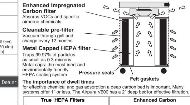
Developed by the atomic energy commission to filter radio active particles as small as 0.3 microns
