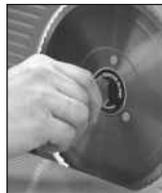
Figure 7. Turn the screw clockwise for blade removal.
