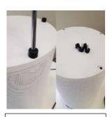
3. USING A SCREWDRIVER REMOVE THE 4 SCREWS
